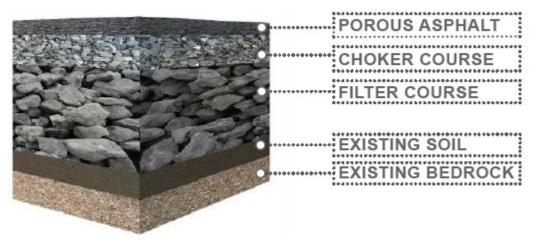
Figure 6: Cross-section of porous asphalt
