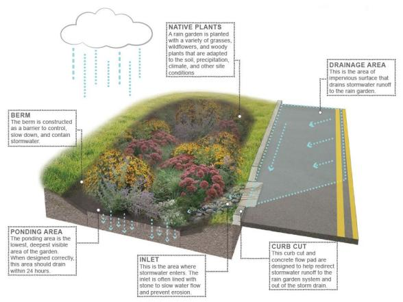
Figure 1: Bioretention system/rain garden
