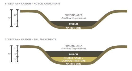
Figure 2: Standard cross-sections of rain gardens
